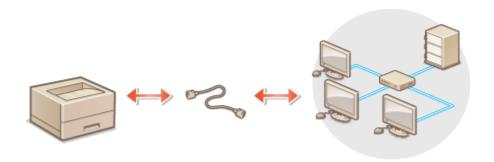
11. 使用區域網路纜線將本機連接到路由器,推入接頭,直至聽到喀嗒聲,開啟印表機 Connect the machine to a router by using a LAN cable, and push the connector in until it clicks into place, and then turn on the printer
