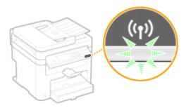
11. 設定完成時,會顯示以下畫面,約 2 秒後 Wi-Fi 指示燈隨即亮起。(When the setup is completed, the screen below is displayed, and approximately 2 seconds later, the Wi-Fi indicator lights up.)
