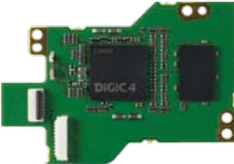
測光系統專屬DIGIC 4處理器 Dedicated DIGIC 4 digital image processor
