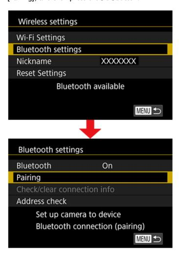
9. 螢幕顯示相機正在等候連接的畫面。 A screen is displayed indicating that the camera is waiting to connect.
