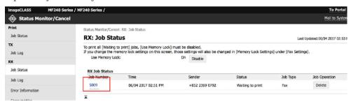
ii. 刪除所有不需要的文件後將記憶鎖定功能轉為[停用],記憶體內的所有文件即會自動列印(列印完成後可再次將記憶鎖定功能〔開啟))。After delete all useless document in Remote UI, all documents in printer will print out automatically by click [Disable] button under memory lock(User can turn the memory lock function [ON] again after all documents printed).
