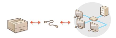
10. 使用區域網路纜線將本機連接到路由器,推入接頭,直至聽到喀嗒聲,開啟印表機 Connect the machine to a router by using a LAN cable, push the connector in until it clicks into place, and then turn on the printer
