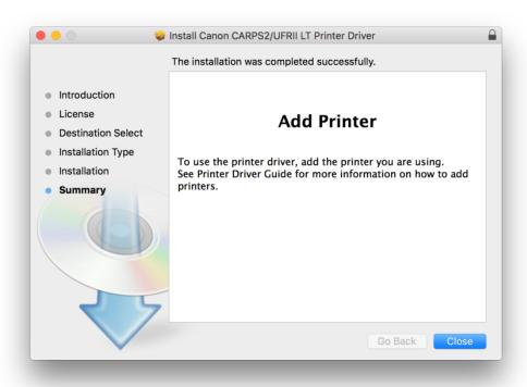
9. 完成安裝驅動程式後需新增印表機,請使用USB線連接印表機與電腦並啟動印表機,再按一下電腦左上角< > 圖案,選擇<系統偏好設定>,再選擇<印表機和掃描器> After finished the driver installation, connect the USB cable with printer and computer, turn on the printer, and please click the top left corner of the computer < i > icon, click < System Preferences>, and then click < Printers and Scanners>
