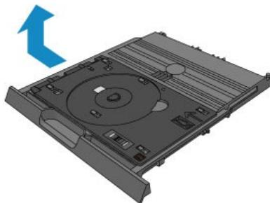
3. 握持出紙托盤(A)兩側，輕輕將其開啟 (Holding both sides of the paper output tray (A), gently open it)
