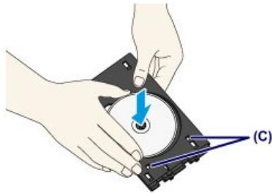
6. 將光碟托盤安裝到本機 (Attach the disc tray to the machine)
