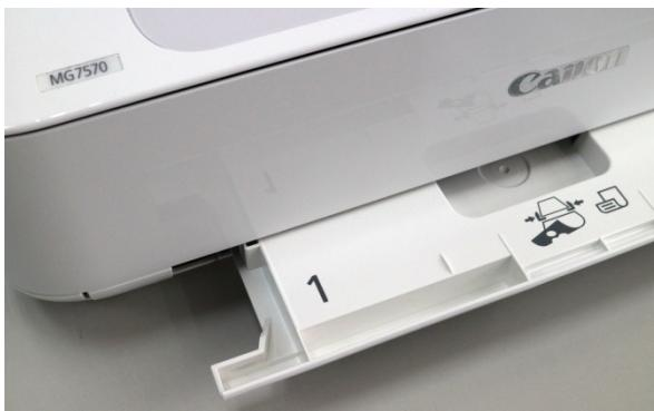
2. 將光碟托盤滑動至紙匣 1的後側，然後將其抬起以取下 (Slide the disc tray to the side on the back of the cassette 1 and raise it to detach)
