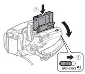
1 Slide OPEN/EJECT fully in the direction of the arrow and open the cassette compartment cover.
