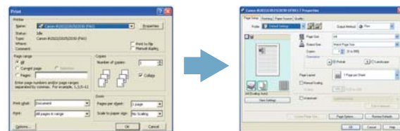
Select [Print] from the file menu → select the fax driver → press [OK]
